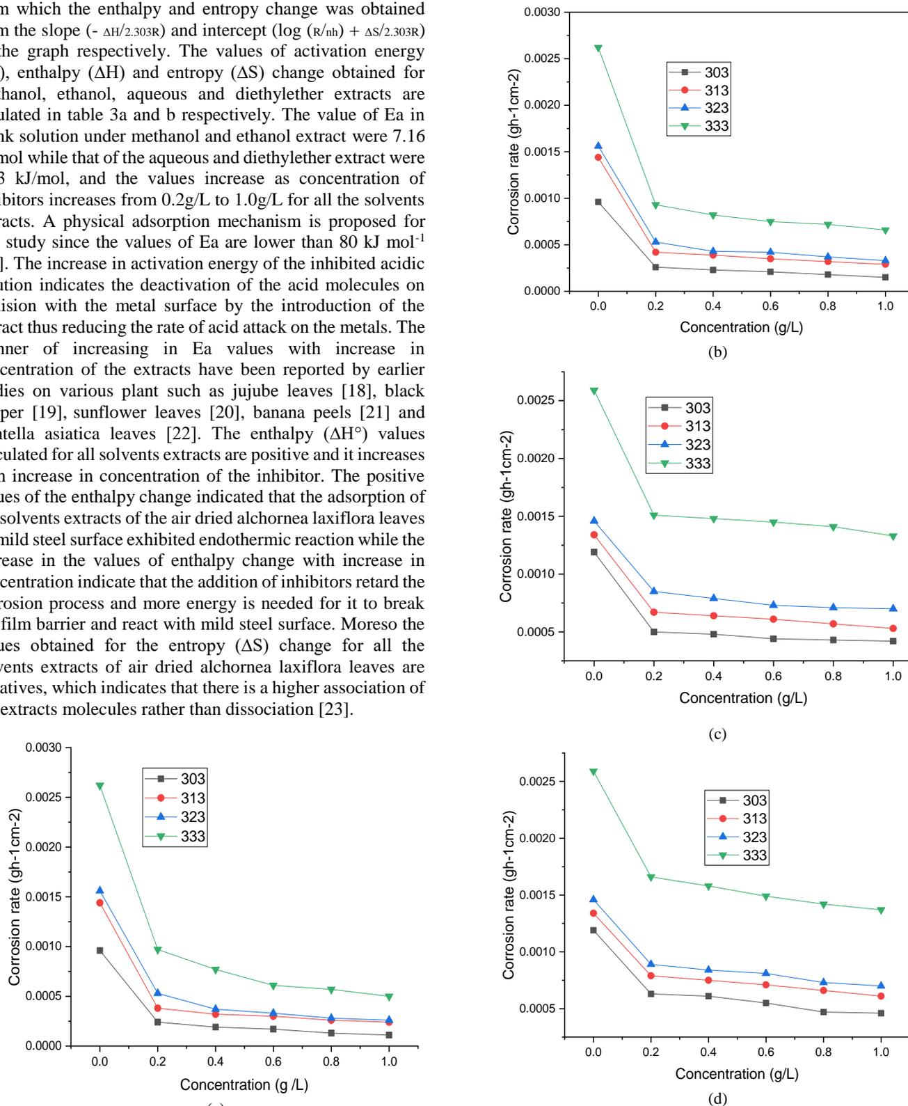
Figure 1: plot of corrosion rate of mild steel against Concentration of (a) Methanol extract (b) ethanol extract (c) aqueous extract (d) diethylether extract at different Temperature
