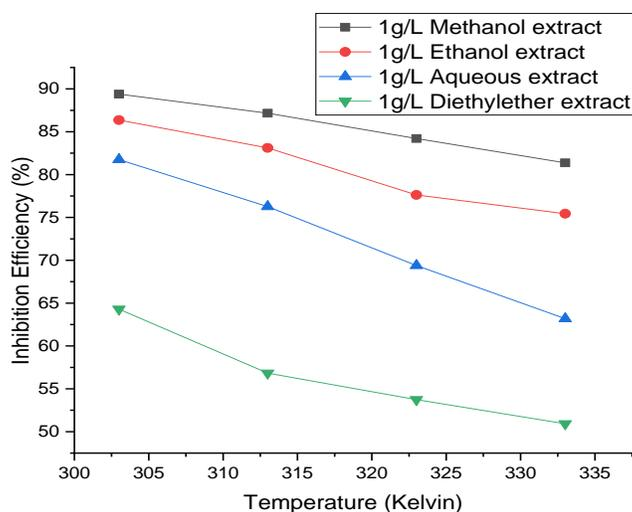
Figure 3: Plot of inhibition efficiency of the solvents extracts against Temperature at fixed concentration
